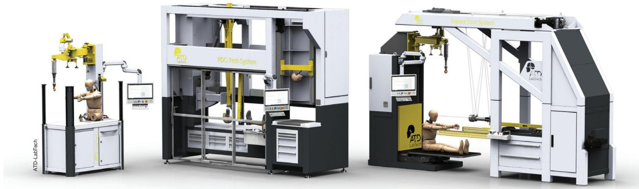
Crash tests are becoming more and more complex. Not only has the testing of single components become more detailed, but more sensors are now needed in full vehicle tests, able to measure to a greater degree of accuracy. This has impacted both R&D and regulatory test procedures. To get comparable results, all 26 types of dummies in use today must be verified in a certification process.
